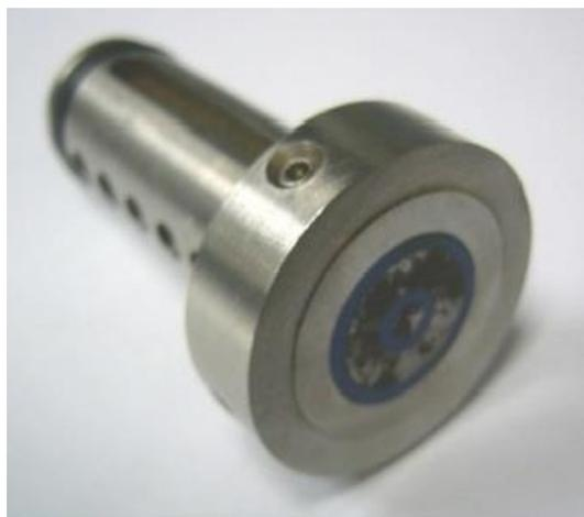
Figure 19: The electrochemical probe used in the mass transfer characterization experiment.
